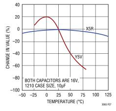
Figure 7. Ceramic Capacitor Temperature Characteristics
