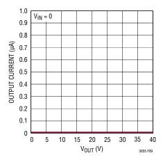
Figure 9. Reverse Output Current
