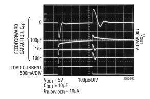
Figure 5. Transient Response vs Feedforward Capacitor
