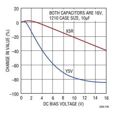
Figure 6. Ceramic Capacitor DC Bias Characteristics
