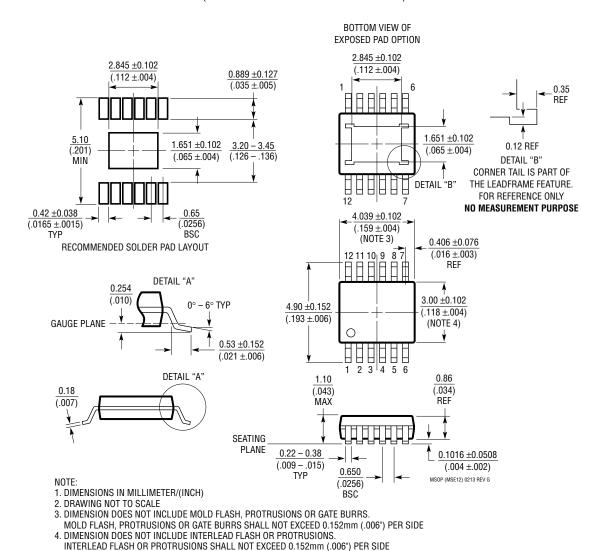
5. LEAD COPLANARITY (BOTTOM OF LEADS AFTER FORMING) SHALL BE 0.102mm (.004") MAX 6. EXPOSED PAD DIMENSION DOES INCLUDE MOLD FLASH. MOLD FLASH ON E-PAD SHALL
