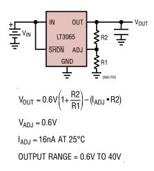
Figure 3. Adjustable Operation
