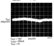
**5V Transient Response**  $C_{FF} = 0$ ,  $I_{OUT} = 50mA$  to 500mA
