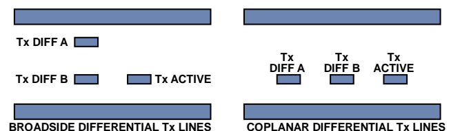
Figure 66. Broadside vs. Coplanar Differential Stripline Routing Techniques
