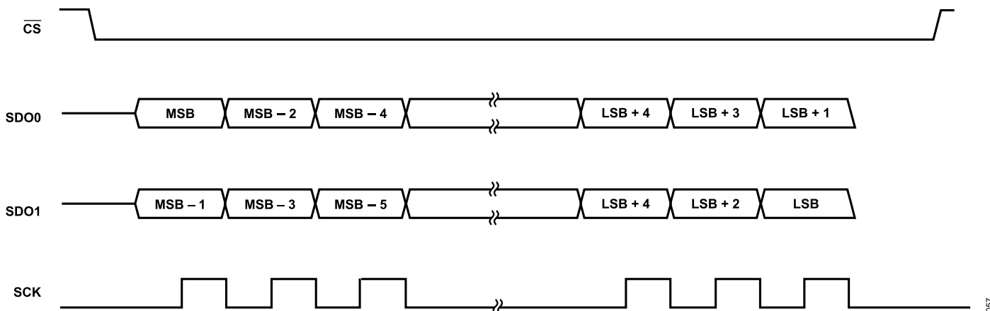
Figure 54. 2-Lane Mode, SDR Timing Diagram
