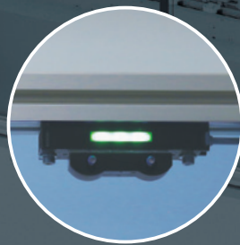
Indicators of other (closed) doors linked to the open door flashes in green to notify unsafe condition.
