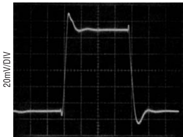
Small-Signal Transient Response V_S = \pm 2.5V
