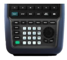
The backlit keypad enables you to use the analyzer in all lighting conditions.
